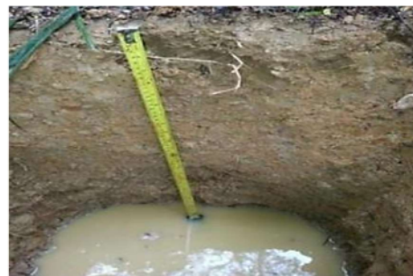
Figure 5. The OB layer is impermeable to water and roots develop in fractures (groundwater table (impermeable) 2-5 years old).
