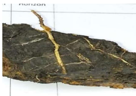
Figure 6. The OB layer is impermeable to water and roots develop in fractures (root growth in cracked, 2-5 years old).
