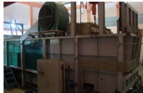
Figure-3. Flume tank and wave generator.
