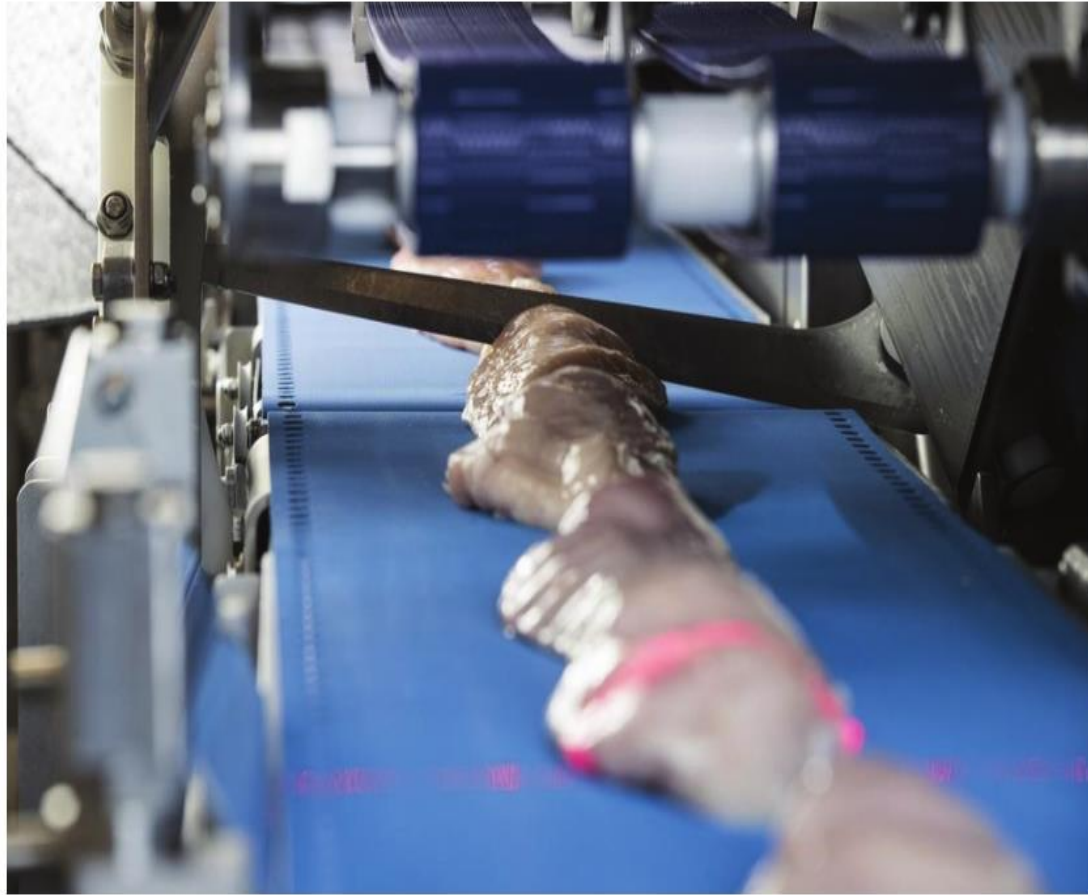
Figure 2. Computer-controlled meat portioning, using automated weighing and laser scanning (see the red line at the front) to get highly accurate target weights at a very fast speed (up to 700 slices/min). Courtesy of Marel.
