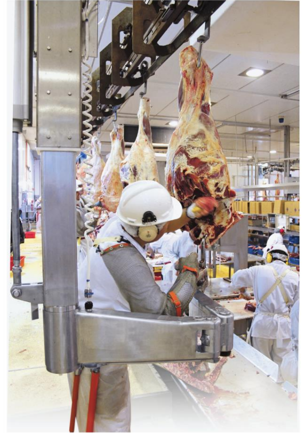
Figure 4. The Beef Boning Unit eliminates the heavy pulling when boning out Beef aitchbones and knuckles.
