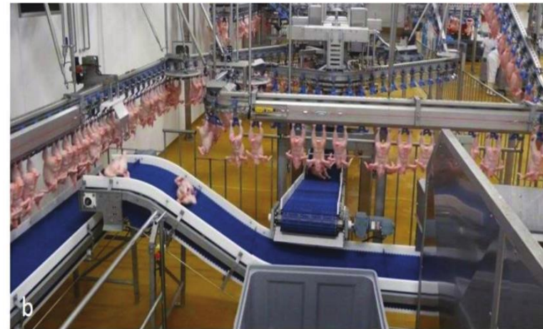
Figure 1. Modern fresh and processed meat plants (a) fully automated forming line, capable of producing 200,000 identical nuggets per hour; (b) in line automated sorting at a fresh poultry processing plant. Courtesy of Marel.
