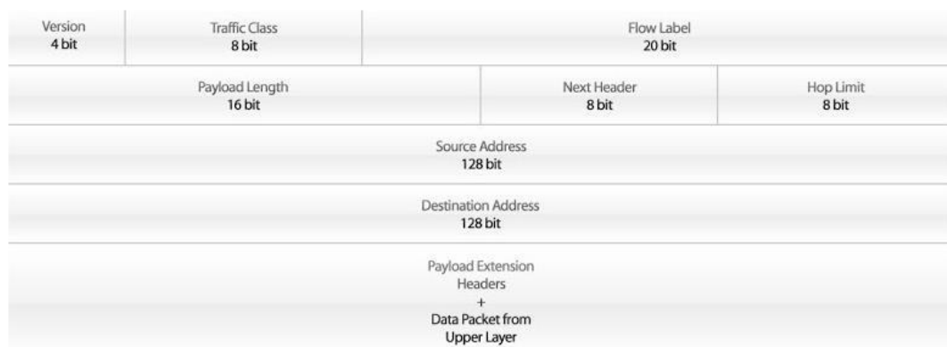
Gambar 4.4 : Format Paket IPv6
