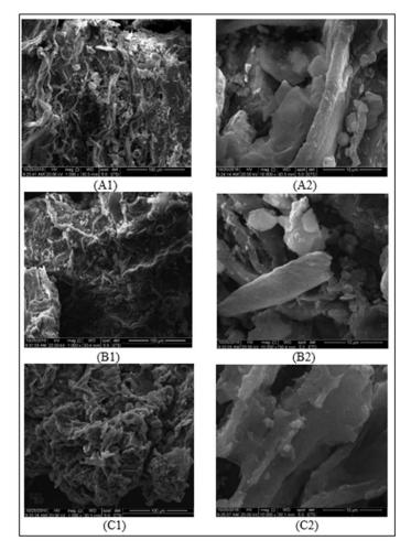
**Figure 2:** Scanning electron micrographs of *P. pellucida* herb samples: (A) Untreated *P. pellucida* sample (A1 is the 100 μm image, A2 is the 10 μm image); (B) after maceration (B1 is the 100 μm image, B2 is the 10 μm image); and (C) after IL-MAE (C1 is the 100 μm image, C2 is the 10 μm image).
