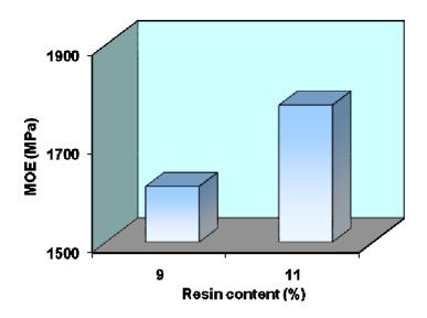
Fig 3: The effect of resin content on MOE
