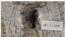
Fig 17- Inside the ground part of control sample is attacked by termites
