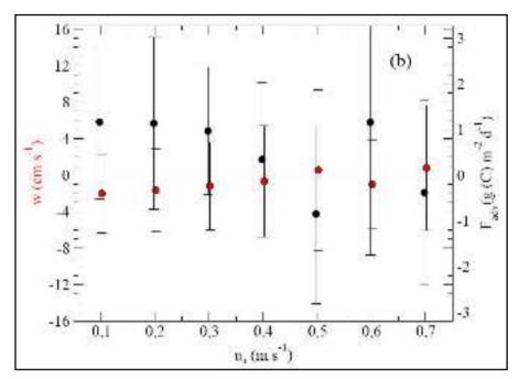
**Fig. 9:** Dependence of Vertical velocity w and Vertical advection  $F_{adv}$  from Friction velocity u\* (Ross, 2007).
