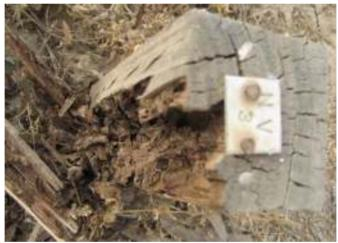
Fig 15- Control samples of *E. viminalis* in Albaji, the attack by termites, and grade No. reached to 0 after 24 month
