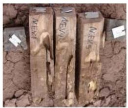
Fig 14- Control samples of *E. viminalis* in Albaji, the attack by termites started after 8 month, and then the grade No. reached to 5.1 after 18 month
