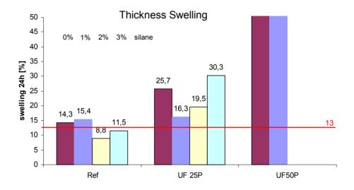
Figure 5: Mechanical technological properties of particle boards produced with modified binding agents – 20 mm particle boards; 200 °C; 3 min; 700 kg/m<sup>3</sup>; glue ratio: 11 % / 8.5 % - *Thickness Swelling* after 24h of water storage
