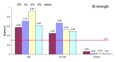
Figure 2: Mechanical technological properties of particle boards produced with modified binding agents – 20 mm particle boards; 200 °C; 3 min; 700 kg/m<sup>3</sup>; glue ratio: 11 % / 8.5 % - *Internal Bonding Strength*
