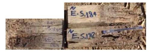
Fig 12- Control samples of *E. striatycalyx*, the attack by termites started after 24 month, then the grade No. reached to 2.4 after 118 month installation inAlbaji and Mishmast station
