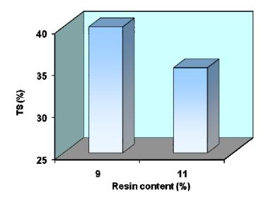
Fig 12: The effect of resin content on T.S. after 24 hours
