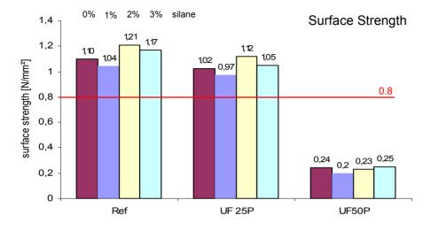
The results for the testing of the surface strength properties are shown in figure 3.
