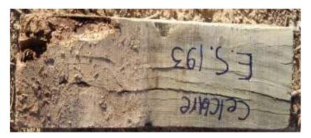
Fig 13- Treated with Celcure samples of *E. striatycalyx*, the attack by termites started after 36 month, then the grade No. Reached to 3 after 96 month installation in Albaji
