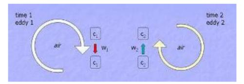
**Fig. 3:** At time 1 eddy 1 transports the concentration c1 downwards with the velocity w1; at time 2 eddy 2 transports concentration c2 upwards with velocity w2. Integration over time gives the net-flux of c (Burba, 2007).
