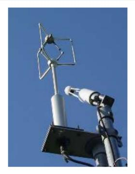
Fig. 2: Ultrasonic anemometer (Campbell CSAT3, left) and infrared gas analyzer (Li-Cor 7500, right) (Burba, 2007).
