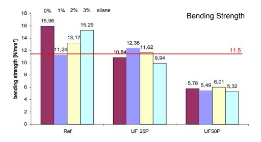
Figure 4: Mechanical technological properties of particle boards produced with modified binding agents -20 mm particle boards; 200 °C; 3 min; 700 kg/m<sup>3</sup>; glue ratio: 11 % / 8.5 % - *Bending Strength*
