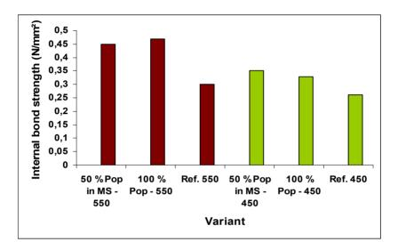
Figure 5: Internal bond strength (N/mm<sup>2</sup>) of the different variants
