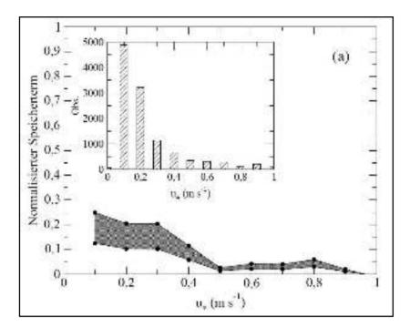
Fig. 10: Normalized storage flux as function of friction velocity u\* (Ross, 2007).
