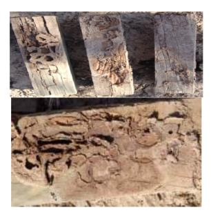
Fig 8-Control samples of *E. camaldulensis* in Albaji and Mishmast station, the attack by termites started after 36 month and then the grade No. reached to 6.7 after 118 month
